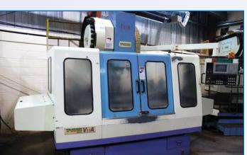
TAKUMI CNC VERTICAL MACHINING CENTER, MODEL V11A
